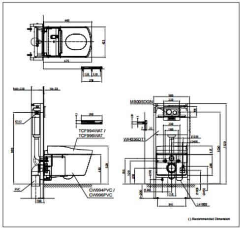
Specifications: Flush System :Tornado Water Use :4.5/3L Rough-in :H = 220mm Water Pressure :0.05Mpa ~ 0.75Mpa Power Rating :AC220 ~ 240V : 50/60 Hz Length of Power Cord :1.0m Size :424W x 679D x 460Hmm Color :White
