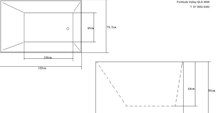
•25mm Profile 8mm Thick Acrylic reinforced with fibreglass
