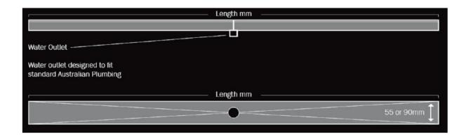
Custom sizes available. Water outlet location, length, depth, etc can all be varied to customer request. A drawing to indicate dimensions & waste outlet location required for all custom orders.
