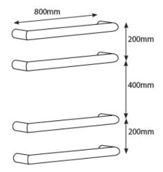
The supplied fixing bracket allows for the above configurations. If more than 5 bars are used an additional fixing bracket will be required.
