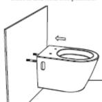
Firmly tighten the Fixing Sleeve all the way into the Fixing Bush Inside of pan.
